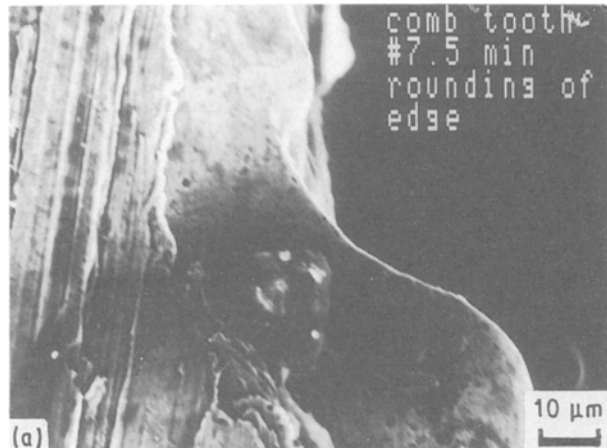
Figure 3 (a) Damage to uncoated comb after 7.5 min testing. (b) Damage to cutter after 6 min testing.
